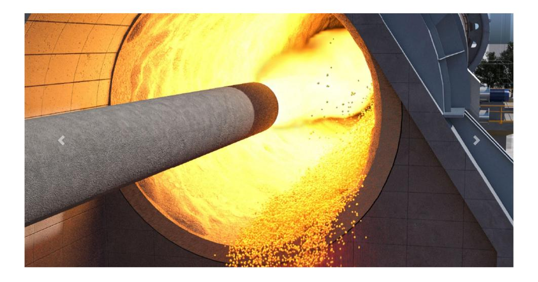
The bottom line: If a plant only ever uses one fuel and rarely switches, for example between coal and natural gas, and current prices do not continue to rise, it makes sense to have two main burners, one for coal only and one for natural gas. But recently, due to rising fuel prices, price volatility and increasing control of cement's CO2 and NOx footprint, many plant operators are demanding a more flexible approach and are increasingly using difficult fuels such as alternative
